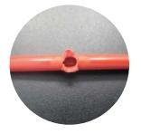
Jactone PAFSS fire suppression systems require no power for detection or operation. PAFSS fire detection tubing is installed throughout the risk area in the workspace, providing fast and effective detection of a fire. Upon flame impingement or high ambient temperature, the pressurised detection tube ruptures with a burst at the hottest point. The extinguishing agent is then discharged via the stainless steel pipework and nozzles which are aimed at the hazard area inside the workspace.
